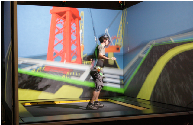
Figure 4: The immersive simulator module of the application prototype running in a CAVE™-like display system setup around an omni-directional treadmill.
